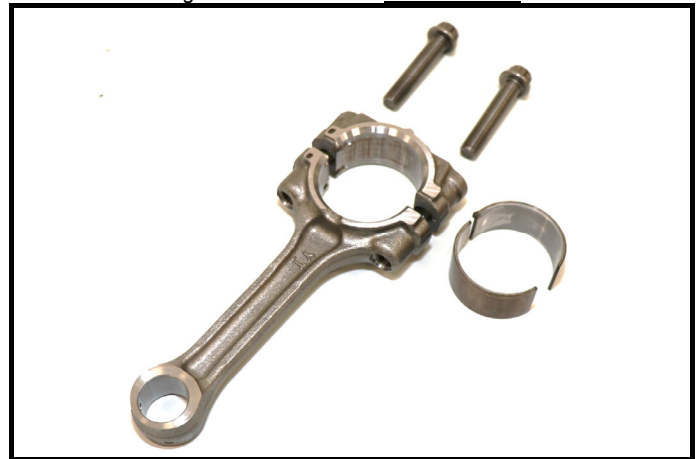
C5-2) Bielle de ¾ arrière côté pied Connecting rod from ¾ rear on small end side
