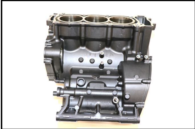
C3-3) Bloc-cylindre nu vu côté droit Bare cylinder block seen from right hand side
