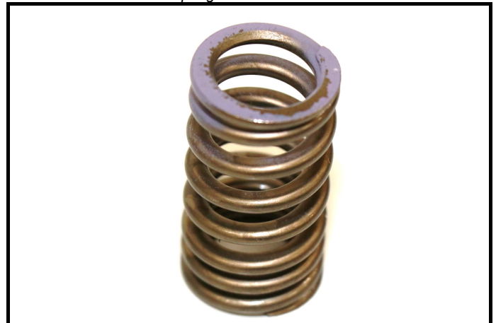
C10-9) Ressort soupape échappement Exhaust valve spring
